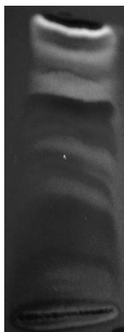
Figure 1. TLC separation of methanolic crude extract of Tolyphothrix sp. using Chloroform: Methanol (4:1) as mobile phase, visualized under UV light 365 nm.
