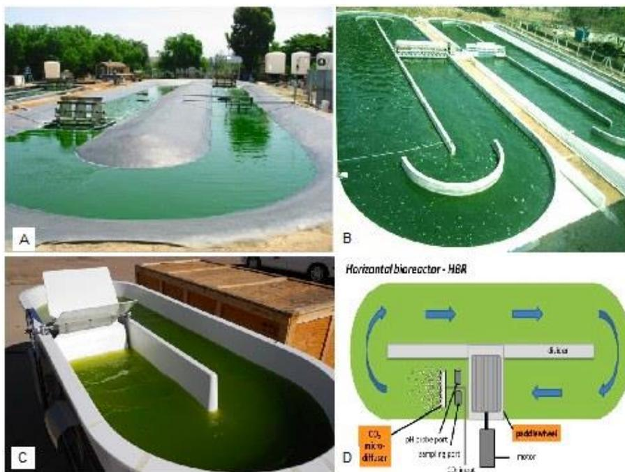
Fig. 1. Open raceway ponds for algal cultivation, A. Raceway pond with thick dividing section (Source- SARDI, South Australia), B. Open raceway pond (Source- Arban Infrastructure Pvt. Ltd., Biotech division), C. Laboratory scale high rate algal pond (Source- New Mexico State University), D. Schematic of the horizontal pond or bioreactor (Source- Brown et al., 2015).
