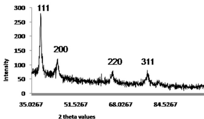
Fig 3 XRD patterns showing 4 peaks of elemental gold
