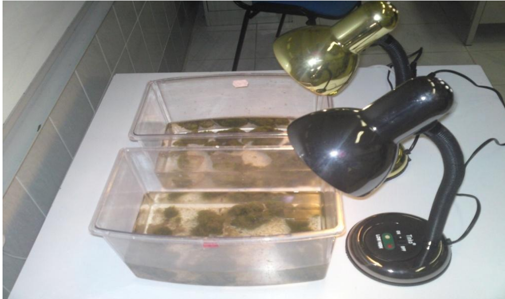
Fig. 1 Algae Biomass in Laboratory Scale Photobioreactor
