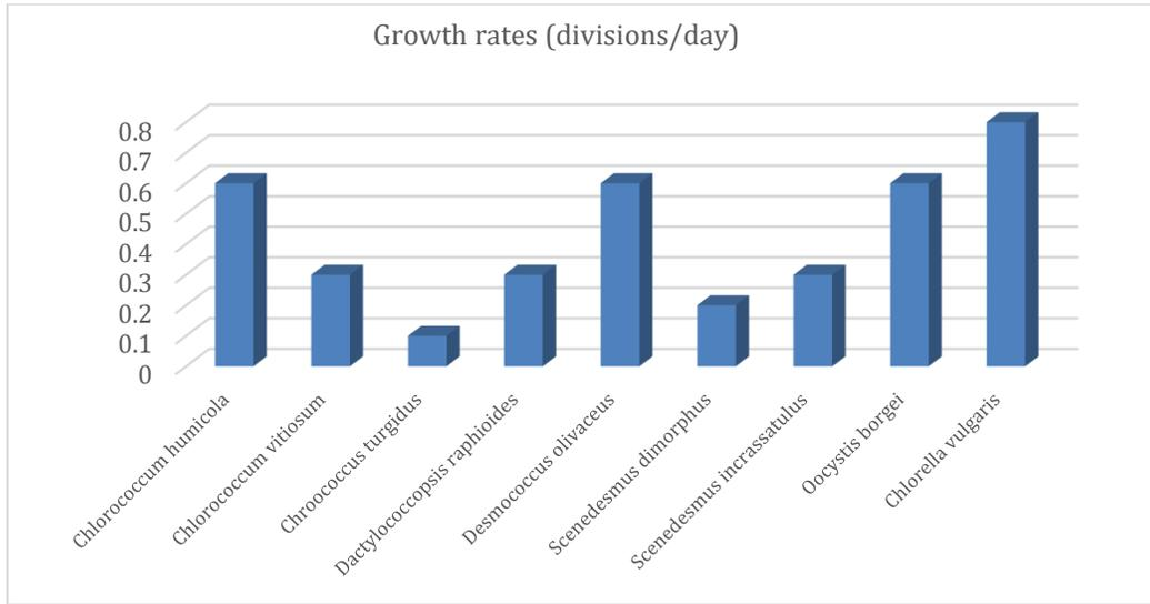
Fig 1. Growth rates of various micro algae grown in R/O reject from a textile industry
