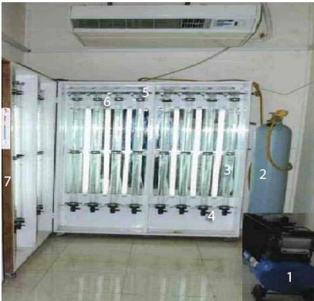
**FIGURE-1:** Principal components of the experimental Photobioreactor prototype. 1-Air generator, 2 - CO<sub>2</sub>source, 3-Glass column 2m height, 4 -Tap for algal growth collection, 5-Air inlet, 6-Air flow adjustment and 7-Thermometer.
